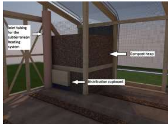
Fig.5: SEG from inside with composting heap.
