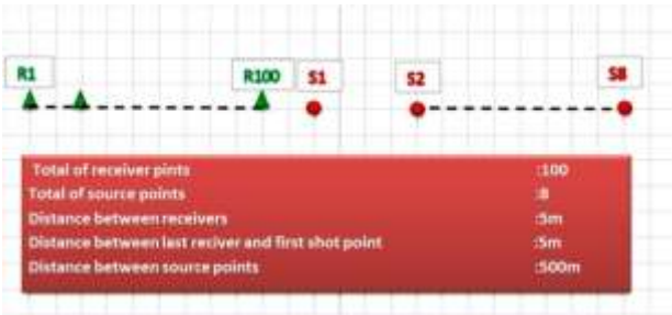
Fig.2: Schematic illustration of distribution pattern for noise test[8].
